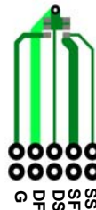
b. 175\text{ }^\circ\text{C/W} when mounted on a minimum pad of 2 oz copper
