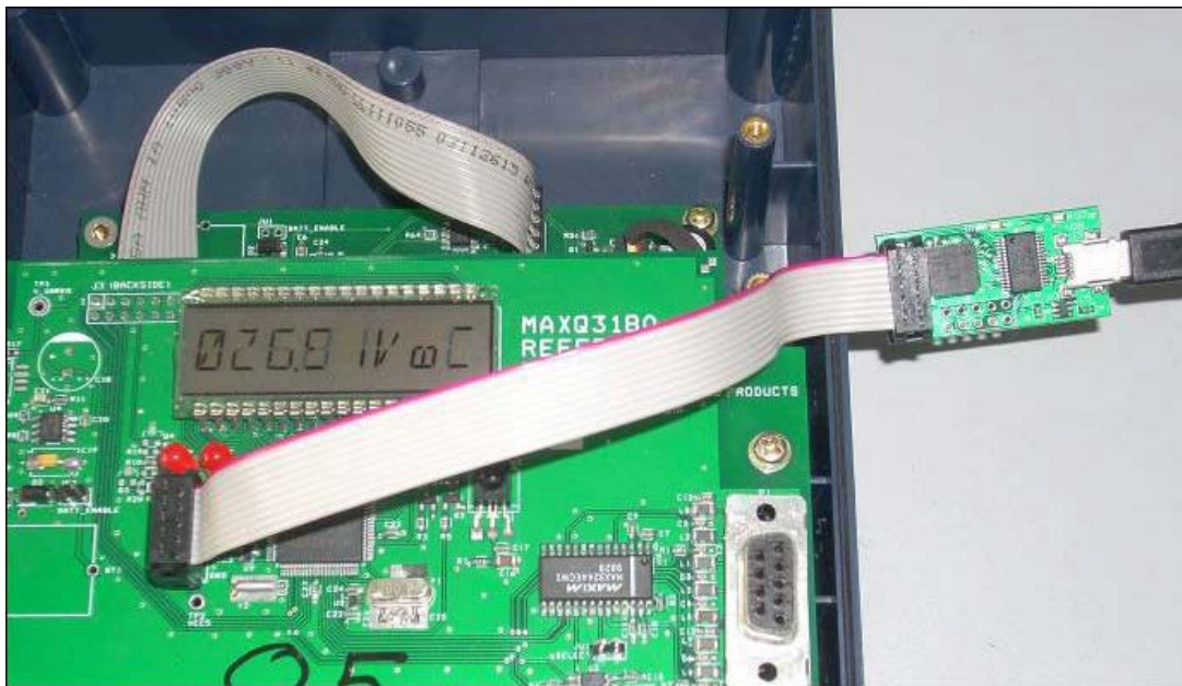
Figure 14. Proper connection of the JTAG cable to the cold board.
