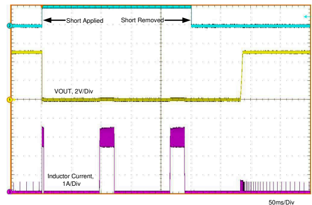
Figure 8-6. Short-Circuit Transient and Recovery
